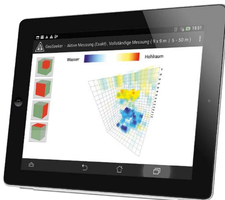
**From the data collected, the GeoSeeker creates an image that shows aquifers and underground cavities.**
